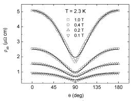
**FIGURE 1.** Resistivity  $\rho_{ab}$  vs angle  $\theta$  measured at 2.3 K. The solid lines are fits of the data with Eq. (3).
